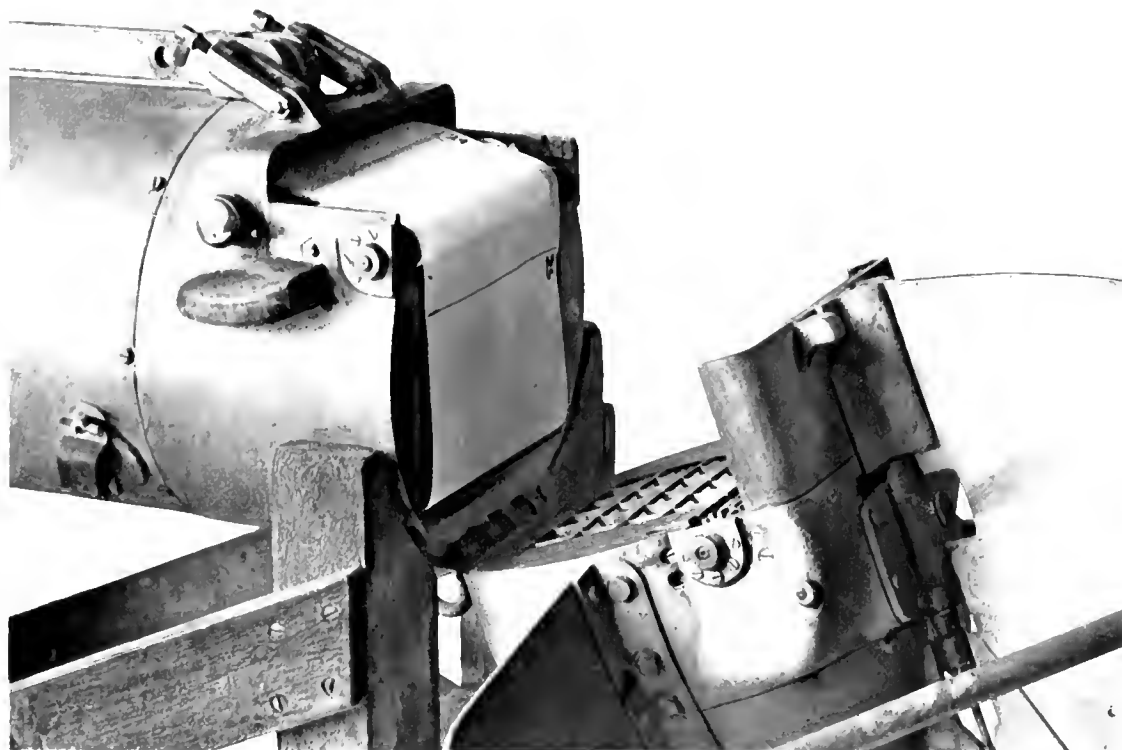
Fig. 2 The Continuous Plankton Recorder, Type I modified, opened to show the gauze bandings in position.
